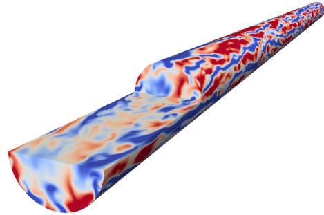
**Figure 1:** Contours of streamwise velocity fluctuations normalized by bulk velocity at bulk Reynolds number of  $Re_b = 5.3 \times 10^3$  (flow direction from right to left).
