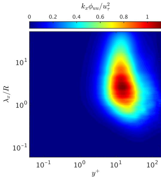
**Figure 2:** Premultiplied energy spectra of streamwise velocity component for turbulent pipe flow at  $Re_b = 5300$ .
