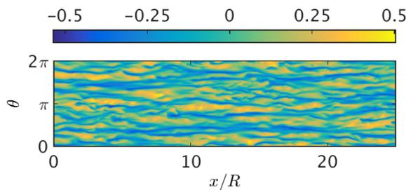
**Figure 3:** Carpet plot of streamwise velocity fluctuations normalized by bulk velocity taken at wall-normal location of  $y^+ = 15$  at  $Re_b = 5300$ . Only  $25R$  of the simulated pipe length is plotted.
