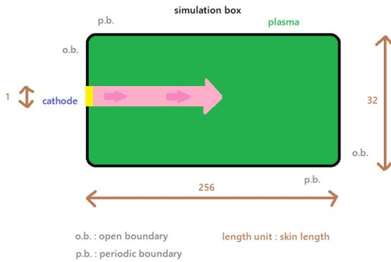
**Figure 2:** Setup of test simulations.
