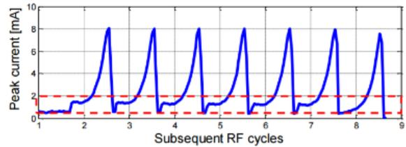
**Figure 1:** Peak electron beam current versus time in units of subsequent RF cycles of the PITZ gun at 1.3 GHz – simulated operation regime optimized for laboratory astrophysics experiments.
