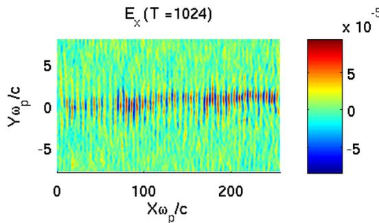
**Figure 3:** Unwanted electrostatic instabilities can provide electric-field noise in test simulations with a bunched electron beam.
