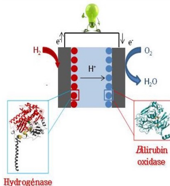
Figure 1: A schematic view of the biofuel cell developed in the BIP Laboratory in Marseille. [NiFe] hydrogenases are adsorbed on the anode, while multicopper bilirubin oxidases are used at the cathode.
