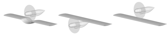
Figure 3: Installation types for the investigation of integrated S-duct intake with actuator disc.
