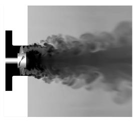
**Figure 1:** Meridional slice of a DES simulation of a low pressure axial fan with the instantaneous density distribution as contour, where brighter areas indicate higher values.
