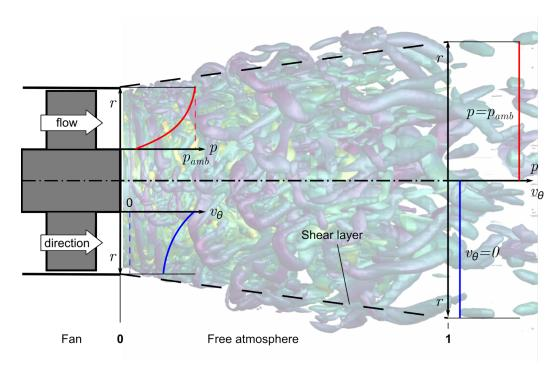
Figure 2: Schematic illustration of the static pressure recovery in the discharge of rotor-only axial fans. From location 0 immediately downstream of the trailing edge of the fan to location 1 far downstream the average static pressure muss increase to ambient pressure.
