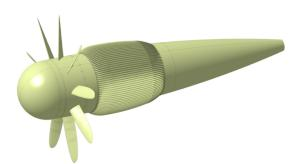
Figure 1: Propeller with heat exchangers placed downstream.
