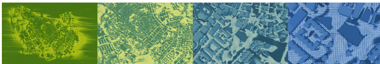
Figure 2: Illustration of the capabilities of PALM-4U: considering meso-scale to micro-scale atmospheric and land-surface processes (frames from left to right) within one and the same simulation, at affordable costs.
