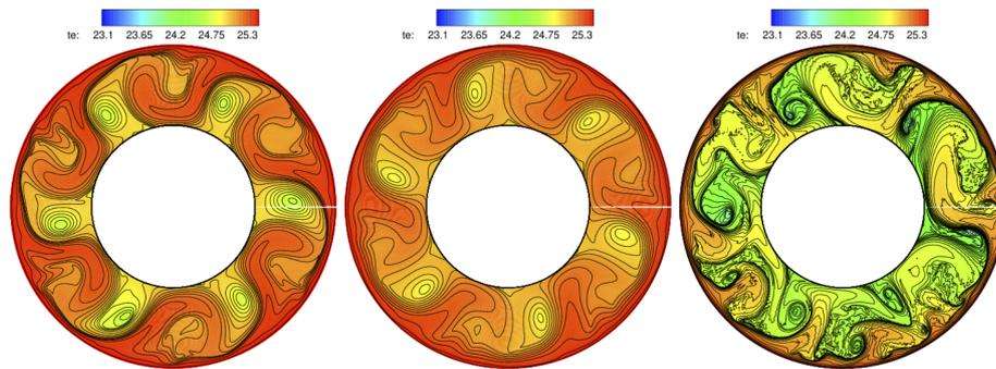
**Figure 2:** Effect of the free-surface model. Snapshots of the surface temperature for several models: adiabatic (left) Marangoni (center) and convective (right).
