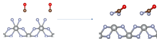
Figure 1: Starting structure for the adsorption of CO on NiF_2 (001) surface and the resulting structure after ionic relaxation.
