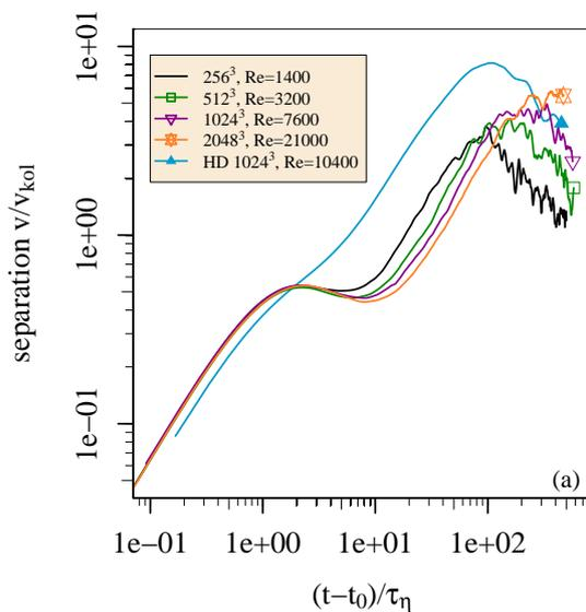
**Figure 2:** Average separation speed particle pairs initially separated by  $2 \eta_{kol}$ , the smallest physical length scale for turbulent motion. Anisotropic MHD simulation run with 8 million tracer particles, for a range of Reynolds numbers and corresponding grid sizes up to  $2048^3$ .
