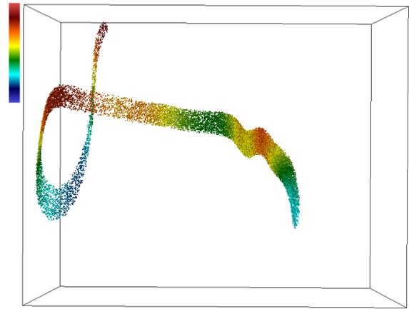
**Figure 3:** A high-density spherical droplet, represented by 16 thousand Lagrangian particles, after dispersing for nearly 40 Kolmogorov time-scales  $\tau_\eta$  in anisotropic MHD turbulence, as described in [4]. Particles are colored by the kinetic energy of the fluid. This is a typical visualization of the ribbon-like dispersion that occurs in these simulations.
