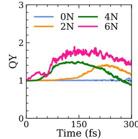
Figure 1: CM QY of graphene with different doping levels. The electron-hole pair is generated by phonon with energy of 3.52 eV at 300K.
