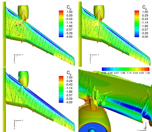
**Figure 1:** Surface pressure distribution, flight Reynolds number at  $\alpha = 16$  deg(top): Coarse mesh(left); Refined mesh(right); Level-D workshop mesh at wind tunnel Reynolds number at  $\alpha = 20.55$  deg(bottom left); Vortical flow in the stall region, non dimensional  $Q$ -criterion iso surfaces ( $Q * MAC^2 / U_\infty^2 = 50$ ) with  $c_p$  contour at  $\alpha = 16$  deg, SA model, refined mesh and flight Reynolds number(bottom right)
